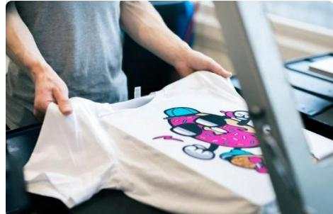
Direct Garment (DTG) printing involves printing designs directly onto fabric using a specialized inkjet printer. The fabric absorbs the ink, creating sharp, high-resolution prints with a soft feel. DTG is perfect for detailed, full-color designs and works best on cotton fabrics. It's ideal for small batches or custom orders, offering flexibility and, importantly, quick turnaround times that enhance productivity.
