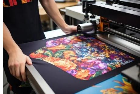
Sublimation printing, a process where heat transfers dye onto fabric, turning the dye into gas without passing through a liquid state, results in vibrant, full-color designs that are absorbed into the fabric. These colors are not only vibrant but also long-lasting and resistant to fading or cracking, making the visual impact of sublimation printing truly exciting. It's ideal for polyester fabrics and is often used for custom sportswear, apparel, and promotional items.
