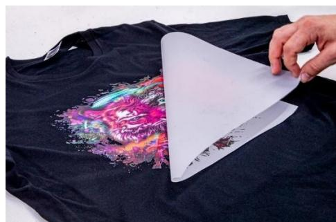
Direct-to-film (DTF) printing is a process that involves transferring digital images directly onto film. This technique is widely used in industries such as apparel printing, particularly for creating custom designs on t-shirts. One of the key benefits of DTF printing is the high-quality and durable results it provides. The digital file is first printed onto a special film, which is then used to transfer the image onto various surfaces.
